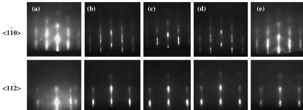
**Fig. 4** RHEED patterns for  $^{107}\text{Ag}/\text{Si}(111)$  prepared with 10 eV (a), 30 eV (b), 50 eV (c), 100 eV (d), and 150 eV (e) ions at the substrate temperature of RT
