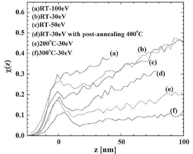
**Fig. 7** Normalized yields vs. depth for  $^{107}\text{Ag}/\text{Si}(111)$  prepared with 100 eV  $^{107}\text{Ag}^+$  ions at the substrate temperature of RT (a), 30 eV at RT (b), 50 eV at RT (c), 30 eV at RT with post-annealing at 400°C (d), 30 eV at 200°C (e), and 30 eV at 300°C (f)
