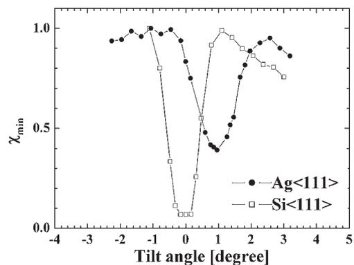
**Fig. 8** RBS-channeling angular scans of the backscattering yield obtained around the Si(111) and Ag(111) axes
