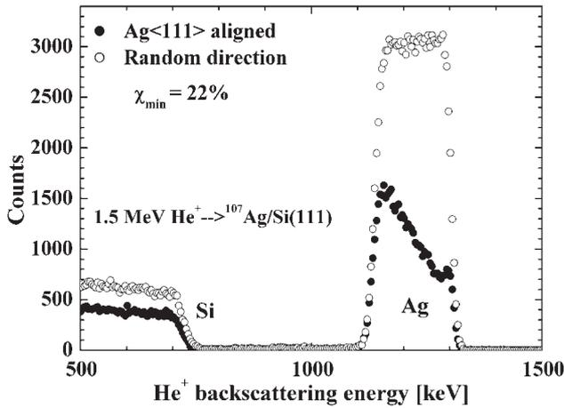
**Fig. 6** RBS-channeling spectra of Ag(111) aligned and random direction for  $^{107}\text{Ag}/\text{Si}(111)$
