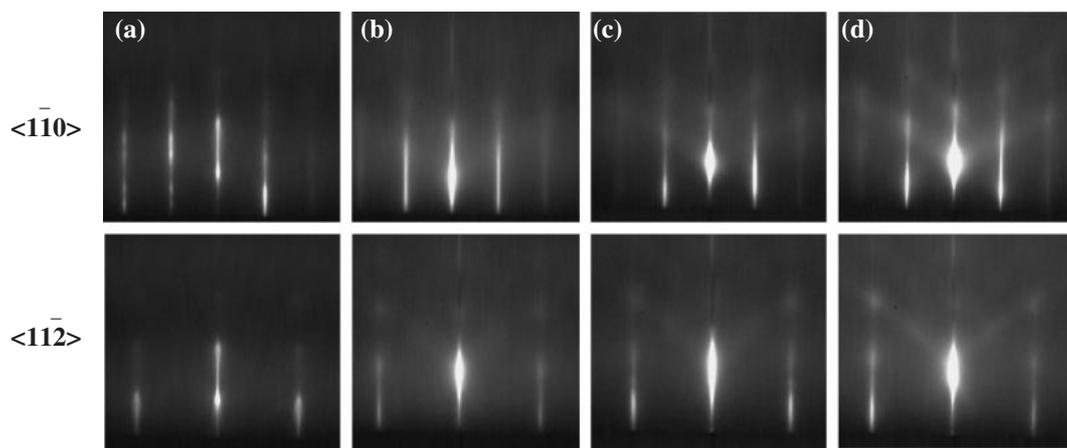
**Fig. 5** RHEED patterns for  $^{107}\text{Ag}/\text{Si}(111)$  prepared with 30 eV Ag ions at the substrate temperature of RT (a), RT with post-annealing at 300°C (b), 200°C (c), and 300°C (d)
