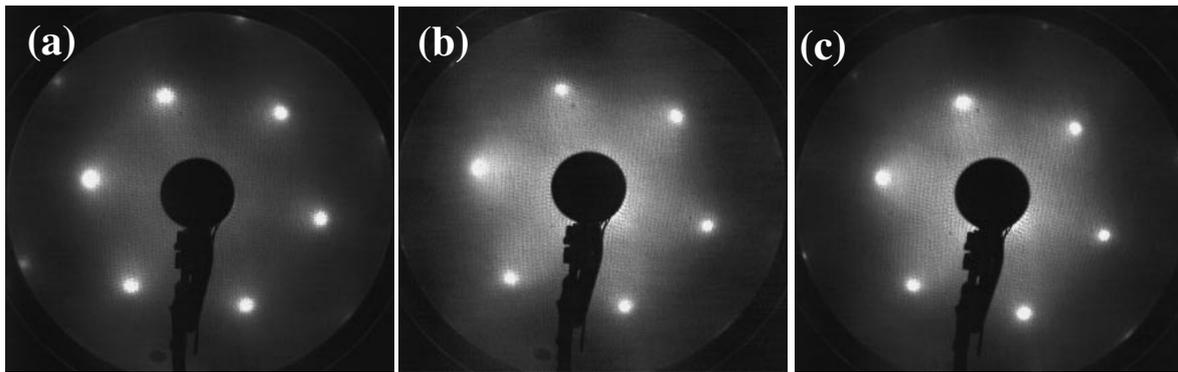
**Fig. 3** LEED patterns ( $E_p=110$  eV) for  $^{107}\text{Ag}$  film/Si(111) prepared with 30 eV  $^{107}\text{Ag}^+$  ions at the substrate temperature of RT (a), RT with post-annealing at 300°C (b), and 300°C (c)
