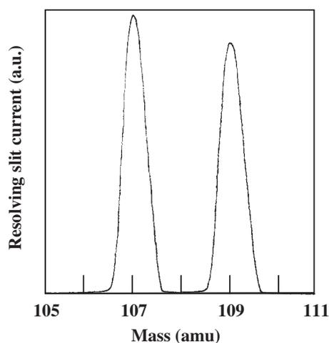
Fig. 2 Mass dependence of the  $\text{Ag}^+$  ion beam intensity
