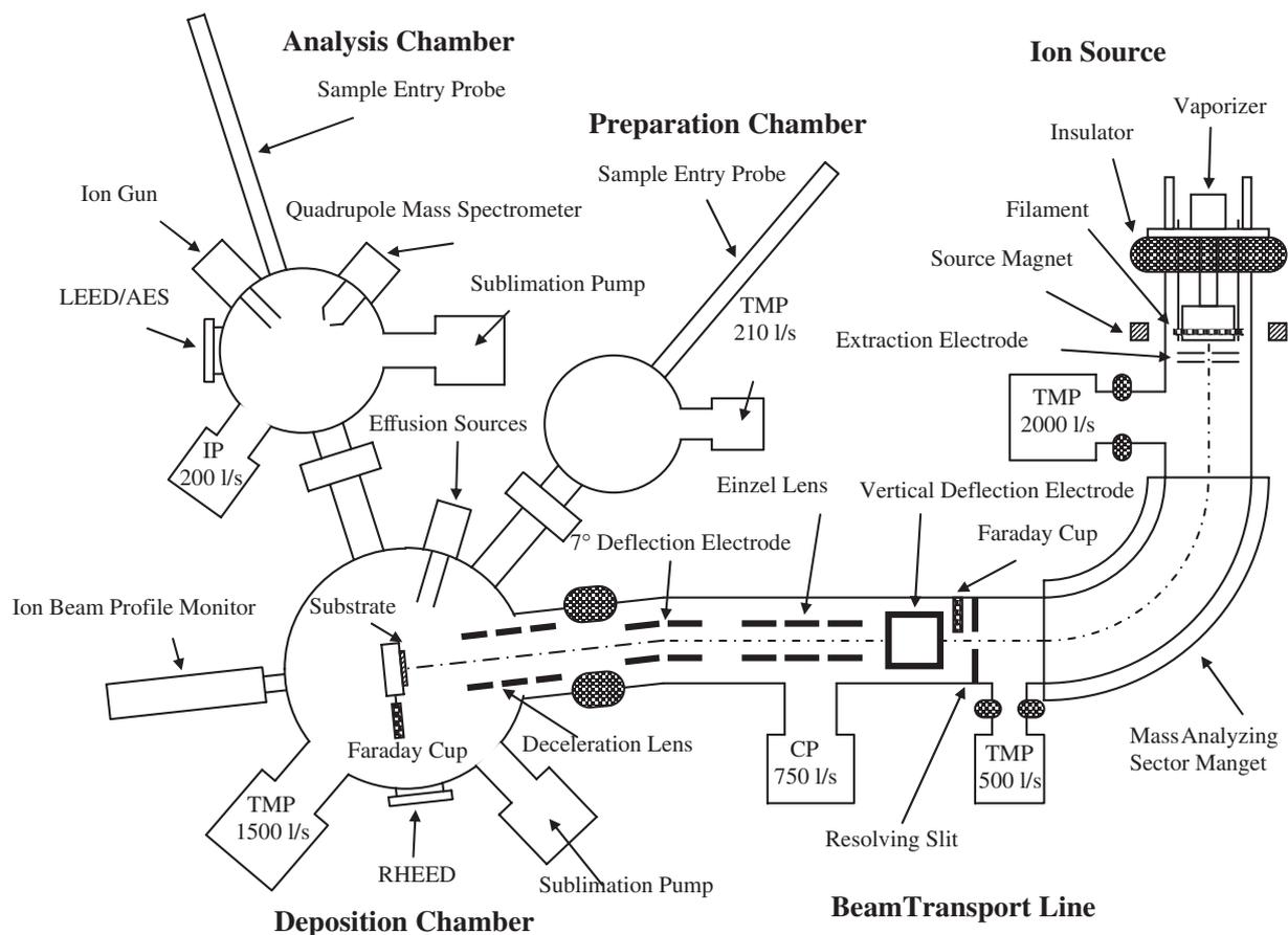
Fig. 1 Schematic illustration of the IBD experimental system
